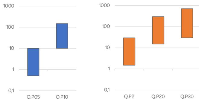
Q.ANT Q.P Particle Sensor configurations. Measurement ranges in  $\mu\text{m}$ , y-axis.
